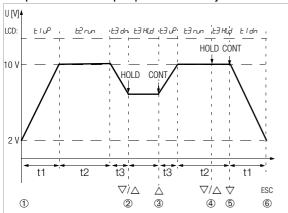
**Ramp parameters:** output quantity: U (range of 0 ... 15 V),  $5 \pm Rr \pm 2$  V, End = 10 V, El = 5 S, El = 8 S, El = 5 S. rEPERE for periodic ramp
