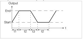
Manually Controlled Ramp Sequence After entering all parameters, start with  $\begin{tabular}{c} \textbf{OUT} \\ \hline \textbf{ENTER} \end{tabular}$  . Rising or falling ramps can be triggered with the \$\triangle\$ or \$\nabla\$ key.
